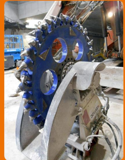
Developed to meet customer requirements, the 1,600 mm diameter cutting wheel of the DMW 130\_600 is fitted with a stabilizer shoe to reach a cutting depth of 500 mm.
