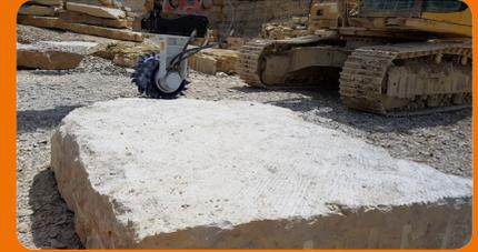
The same raw block after grinding with the KEMROC grinder. It now has a clean surface and greatly improved profile.
