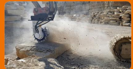
The KEMROC grinder in action. It takes one minute for the excavator operator to completely clean and profile the surface of one block.
