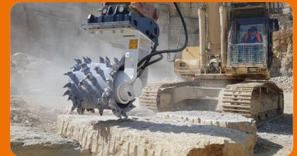
After testing for one week, the quarry purchased a KEMROC ES 60 HD grinder for installation on their own excavator.
