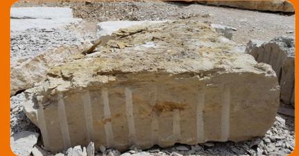
A raw block in Franken-Schotter's Dietfurt limestone quarry. The problematic layer of marl on the upper surface is plainly visible.
