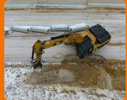
A unique technical feature made it possible to use a chain cutter along a line outside the excavator tracks; as an optional extra, the cutter can be rotated and fixed at an angle to the axis of the excavator arm.
