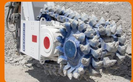
In the KEMROC chain cutter, a patented cutter chain running between two cutter heads is used to get maximum productivity from the available width of the attachment.
