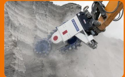
In addition to efficient utilisation of power from the excavator hydraulics, the new production method also uses the weight of the chain cutter to great effect.
