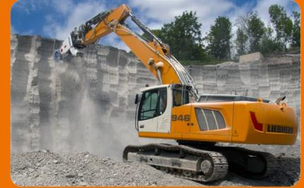
The company Gebrüder Bantle & Co. KG have recently started using a KEMROC EK 140 chain cutter as their primary tool for production at one of the gypsum quarries.
