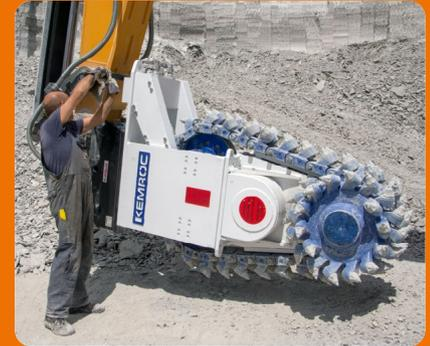
For round attack picks, working in soft material such as gypsum is a very light application. As a result, operating costs in terms of fuel and wear are low.
