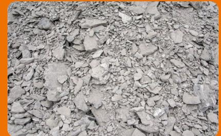
The chain cutter produces a smaller, more consistent grain size material than the hydraulic breaker resulting in savings down the line in crushing costs and material handling.
