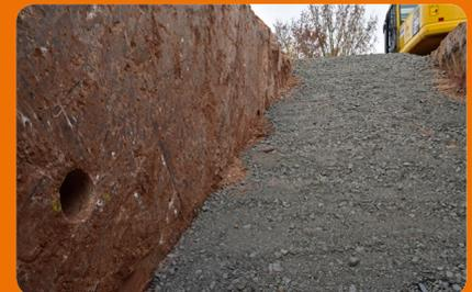
At the KEMROC test site, a completed soil-cement wall is exposed and ready for testing and sampling.
