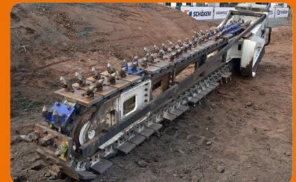
The KSI range of stabilisation attachments are available in different sizes and with a choice of blade length – here the KSI 5000 with 4 m mixing depth before going into operation.
