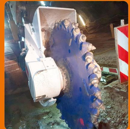
A DMW 130 cutter wheel was chosen with 130 mm cutting width and 600 mm cutting depth.
