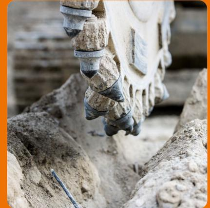
A close-up view of the cutter wheel with round attack picks. In the lightly re-enforced concrete at Konstanz, wear costs were held to acceptable levels.
