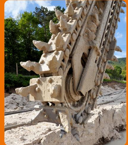
The cutter chain is fitted with exchangeable carbide tipped cutter teeth. Injection nozzles are fitted to the left and right at the front of steel plates on the chain. A semi-mobile mixing plant pumps cement suspension into the ground via hoses to the nozzles on the chain.
