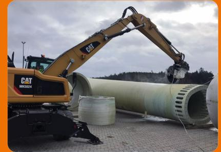
EURECUM uses a Cat MH3024 material handler with a KEMROC KDS 50 diamond saw to cut through wind turbine rotor blades.
