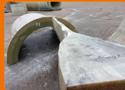
The process developed by EURECUM has proven itself many times in practice. These sections of GRP are ready to be fed into the automated shredding machine.
