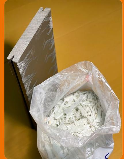
At the end of the recycling process, the final product is a valuable, fine grained material that has a growing number of uses – for decking, as an example.
