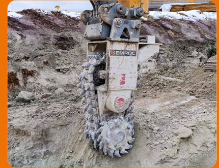
The chain cutter in close up; a chain with tungsten carbide tipped cutters runs between the cutter drums, removing the ridge of rock that normally would be left.
