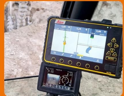
Technicians from KEMROC trading partner Beuthauser installed a GPS control system in the excavator cab. This helped the operator excavate trenches to centimetre tolerances.
