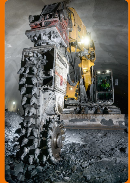
A rotating cutter chain with tungsten carbide tipped picks is the essential feature of Kemroc chain cutters. It enables rock to be removed without leaving any residue.
