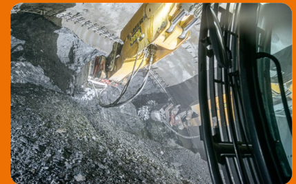
Porr also uses a standard rotary drum cutter. It proves advantageous for certain work areas.
