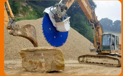
A KEMROC ES 110 HD universal cutter (110 kW) with cutter wheel (1,000 mm cutting depth) mounted on a 24-ton excavator at Fark Naturstein in the Münster region of Germany.
