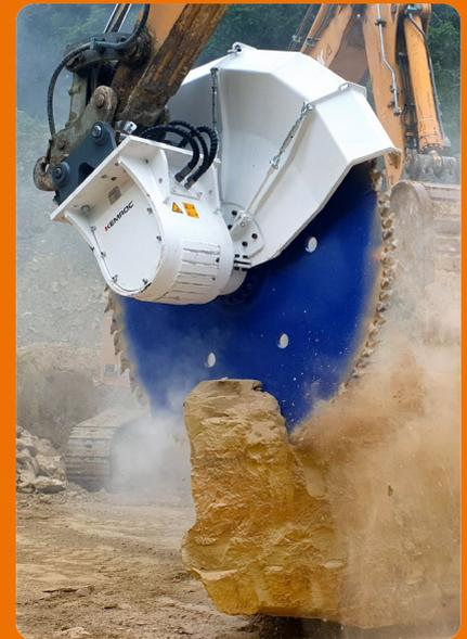
Sandstone blocks can be dressed into manageable sized blocks quicker, better, and more conveniently than by the drilling and splitting method used before.
